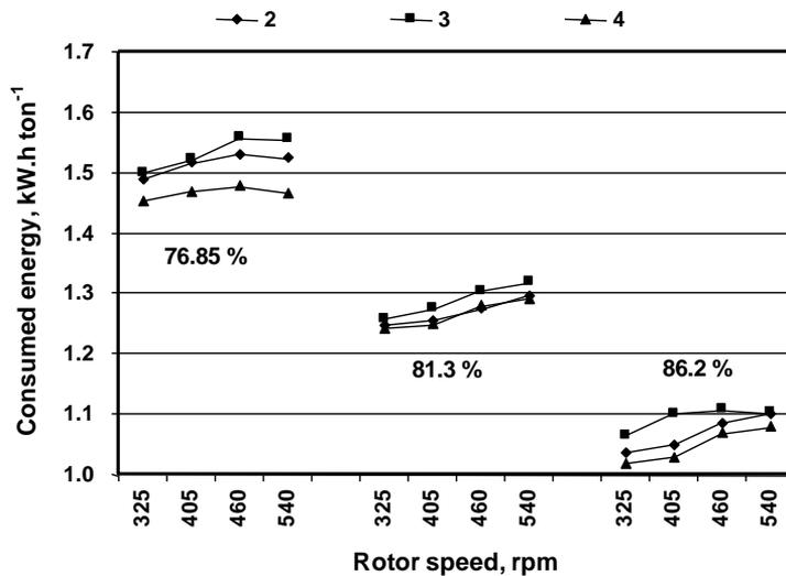
Fig. (12): The effect of moisture content, number of knives rows and rotor speed on the consumed energy.
