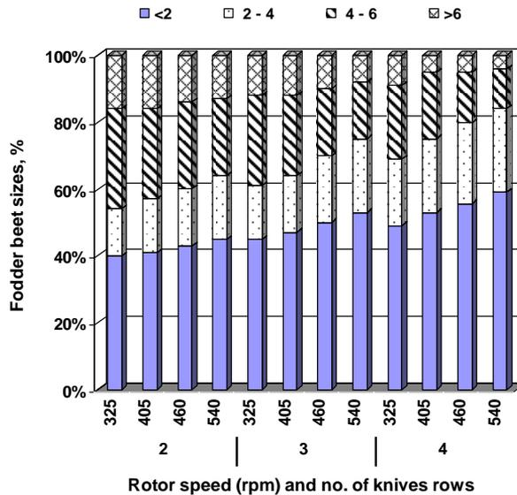
**Fig. (8): The effect of number of knives rows and rotor speed on the beet size at 76.85 % moisture content.**
