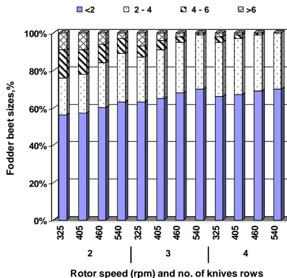
**Fig. (10): The effect of number of knives rows and rotor speed on the beet size at 86.2 % moisture content.**
