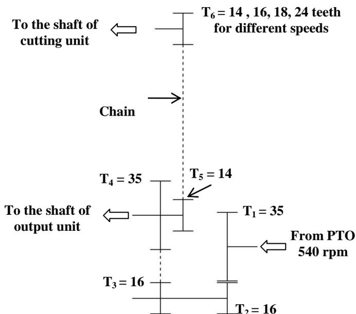
**Fig. (7): Transmission system of modified machine.**
