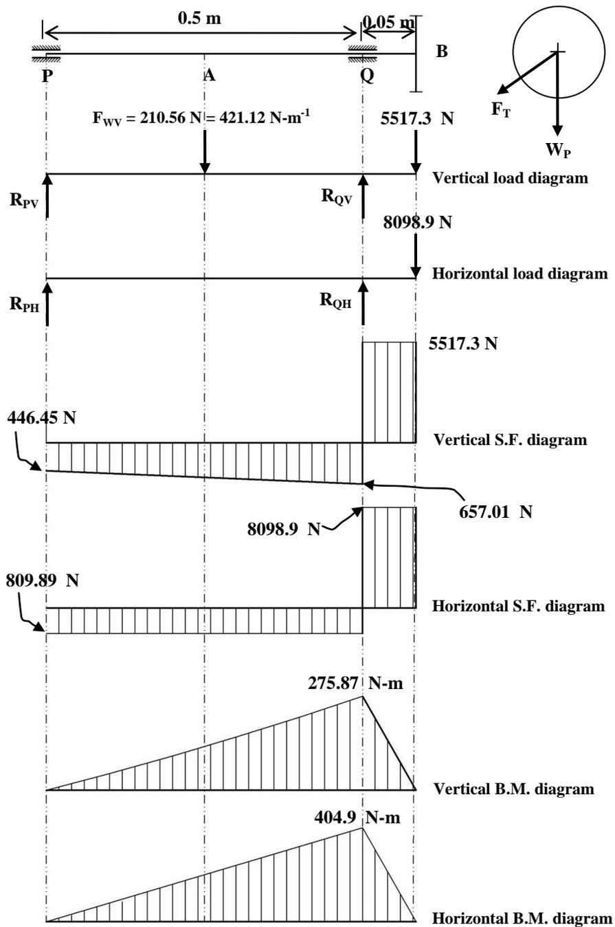
Fig. (6): The shearing and bending moment diagrams of the shaft.
