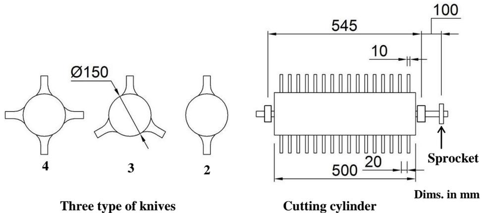
**Fig. (5): Cutting cylinder and shaft of cutting unit.**
