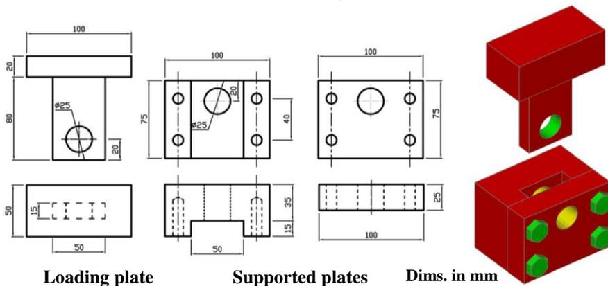
**Fig. (3): The shear force measuring device.**
